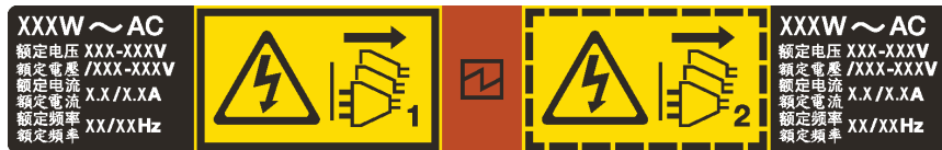
Figure 199. Hot-swap power supply label on the cover
