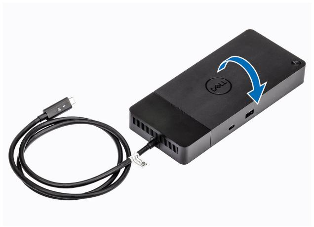
**2.** Remove the two M2.5 x 5 screws [1], and turn over the docking station [2].
