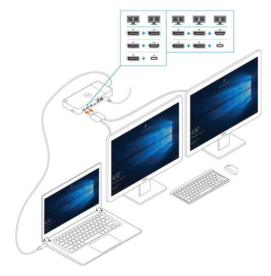
Figure 8. Connecting the multiple displays
