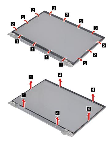
When installing: Ensure that all the latches are attached firmly.
