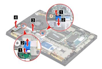
When installing: Ensure that the connectors are attached firmly.
